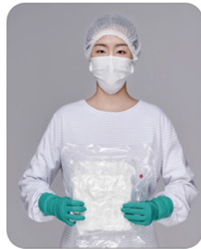
01 Put on the first pair of sterile gloves, face mask and bouffant cap.
