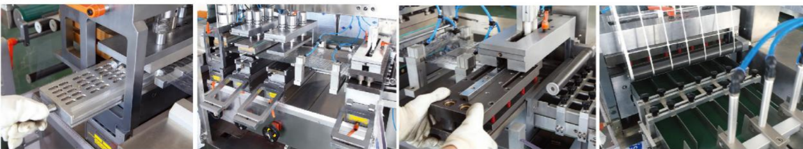
▲ Change mould without tool ▲ Open frame of mould changing ▲ Change punch mould without tool ▲ Blister output device
