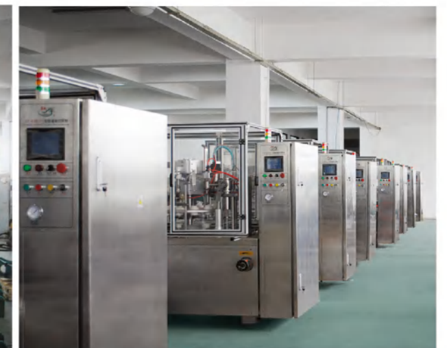
■ Tube filling and sealing machine workshop
