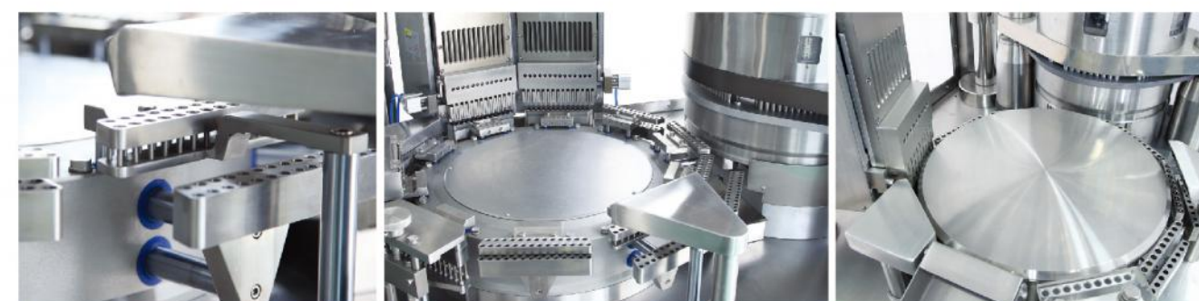
▲ Capsule up and down mould blocks
