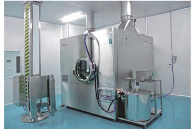
LDB Coating Machine with a Lifting Machine
