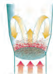
Drying Process ( Drying & Mixing )
