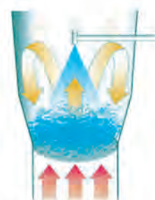
Top Spray Process ( Granulation )
