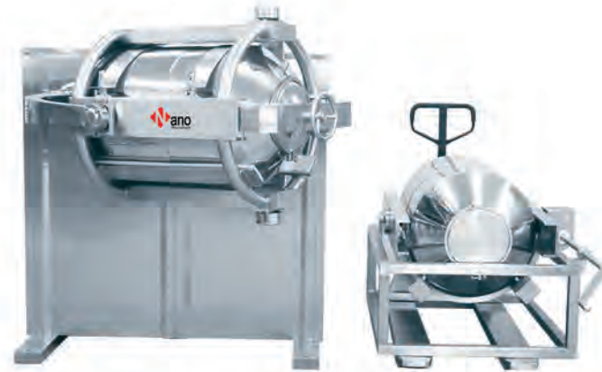
Model HGH 3-Dimensional Blender with Interchangeable Drum
