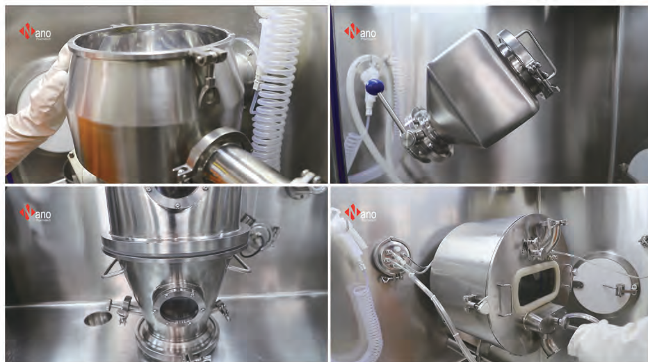
Containment Isolation Granulation System The system consists of Model GHL high shear granulator, Model FL fluid bed granulator, Model KZ/SKZ mill and Model SRH lab blender.
