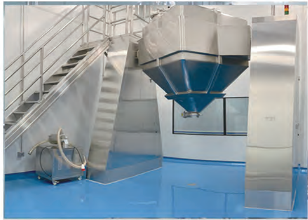
HF Blender with Vacuum Charging System
