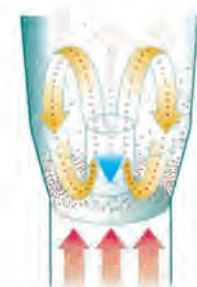
Bottom Spray Process ( Wurster, Coating )
