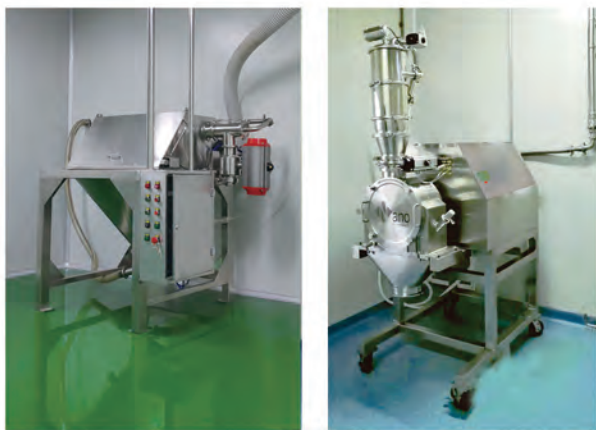
CDZ Bag Dumping Station and CF Hammer Mill
